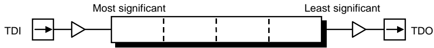
Fig. 23-4 Direction of a Shift of the Instruction Code to the Instruction Register
